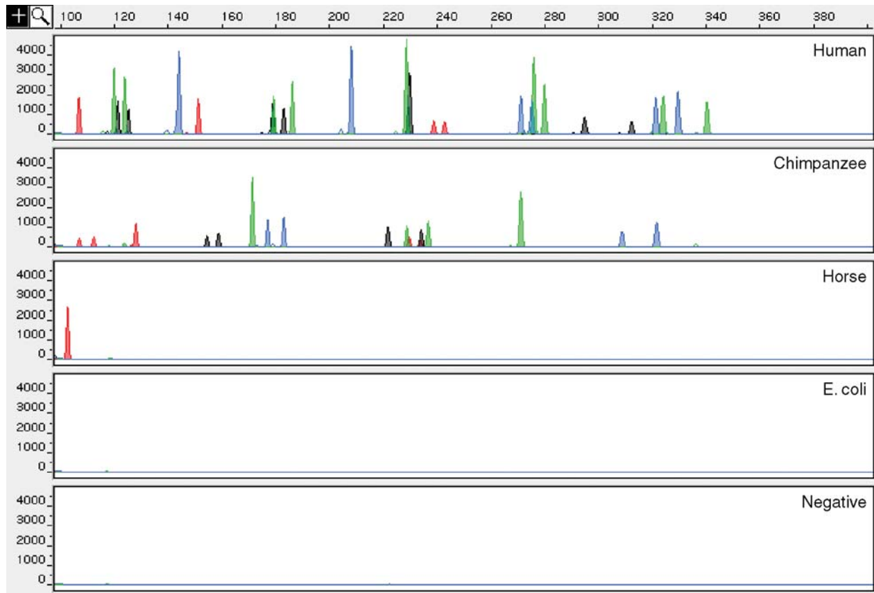
FIG. 3—Representative results from a species specificity study including positive and negative controls. The top panel shows a 1 ng amplification of AmpF \ell STR Control DNA 9947A, panel 2 chimpanzee (1 ng), panel 3 horse (2.5 ng), panel 4 E. coli (5 ng), and the bottom panel the negative control. The X-axis indicates base pair size and the Y-axis RFU. Except for the monomorphic, Amelogenin-like product seen in panel 3, amplification was only observed for primates among all tested species.
