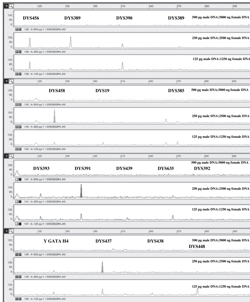
FIG. 3—Varying amounts of male DNA added for amplifying a 1:10,000 male-female mixture. The 250 pg amplification yielded the most genetic information using a 5-sec injection.
