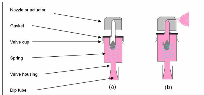
Figure 2. Internal arrangement of a paint spray can
