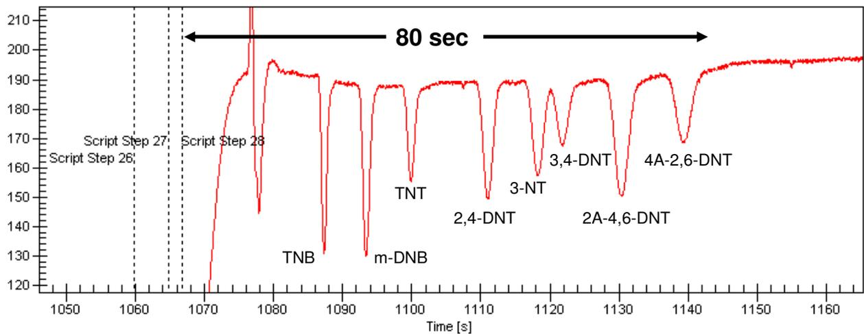
**Figure 4: Separation obtained using an Agilent Bioanalyser 2100 platform. Electrolyte: 50mM SDS & 50mM Borate with 1.5% Agilent™ Dye (v/v).**
