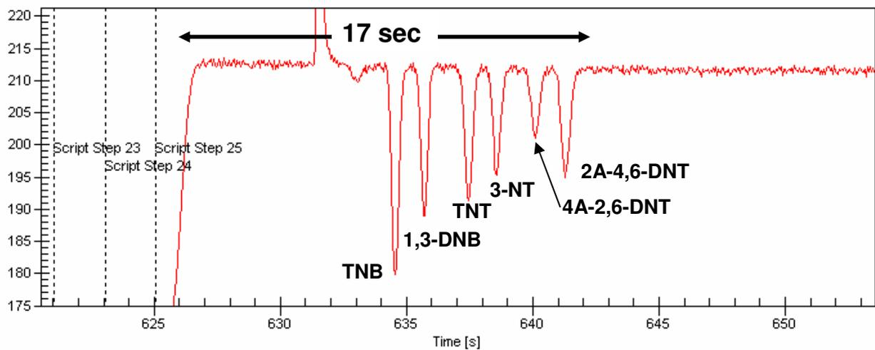
**Figure 5: Separation obtained using an Agilent Bioanalyser 2100 platform. Electrolyte: 50mM Borate & 25mM SDS with 1.5% Agilent DNATM Dye (v/v).**
