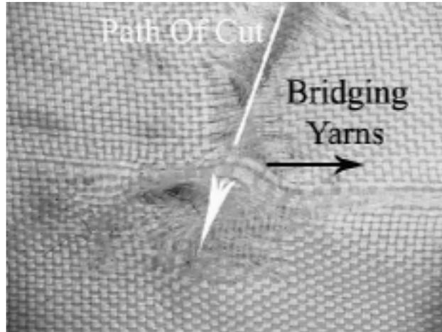
Figure 6 – Cut yarns bridged by uncut yarns.
