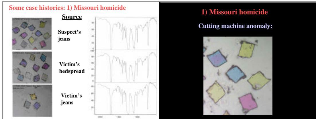
*Notice one corner tends to be rounded and an adjacent corner tends to have a protrusion.*
