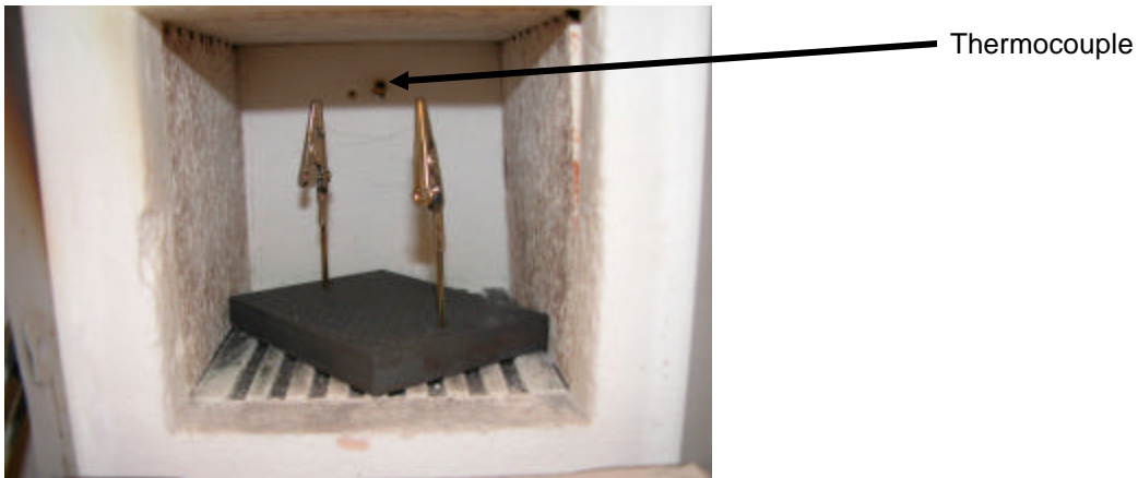
Figure 3: A photograph of the apparatus inside the oven for Study 3. The diagonal orientation of the metal block and the test hair with respect to the oven walls and thermocouple is shown.
