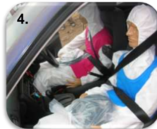
4. Dummies dressed in t-shirts and weighed down, left in-situ during deployment
