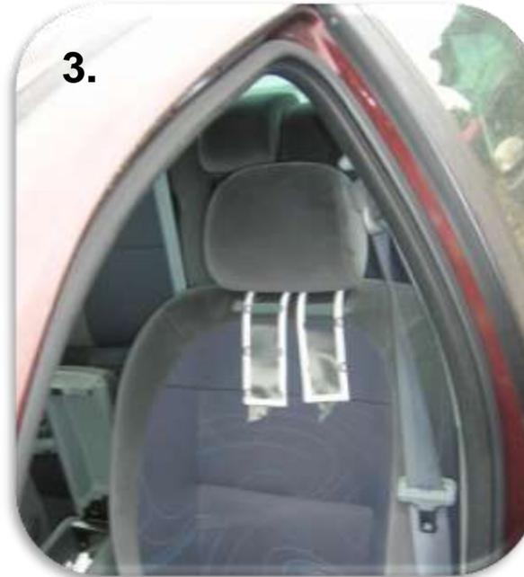
3. Open tape lifts on back of driver and passenger seats, left in-situ during deployment
