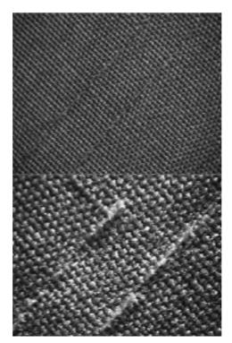
Figure 1 - Parallel cuts in woven fabric.
