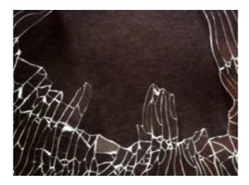
Figure 4 – A broken tempered glass window.
