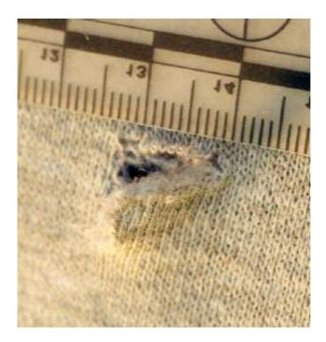
Figure 10 – Glass tear in knit fabric.
