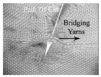
Figure 6 – Cut yarns bridged by uncut yarns.
