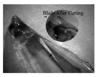
Figure 3 – Magnified view of a glass shard.
