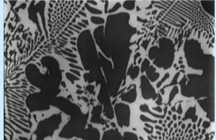
Al-Cu alloy. Copper has a larger nucleus so Cu rich areas appear white, Al rich areas, dark gray.
