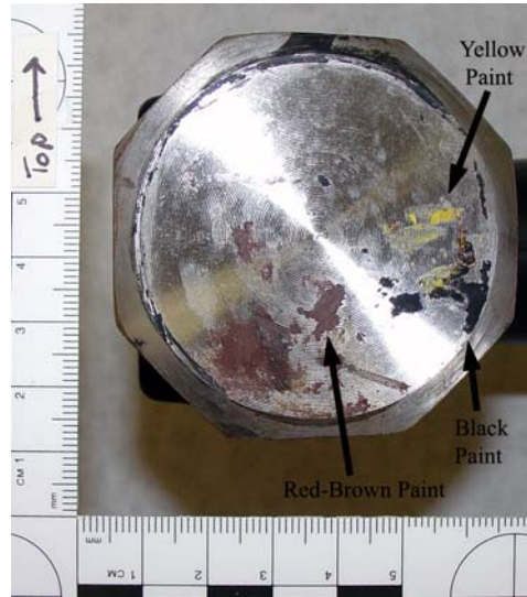
Figure 10. Paint observed on the sledgehammer.
