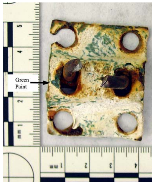
Figure 4. Green paint on u-bolt assembly.
