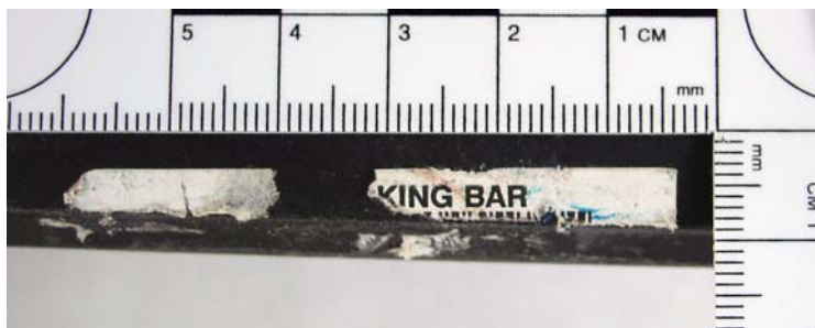
Figure 2. Bar code remnants on suspect pry bar.
