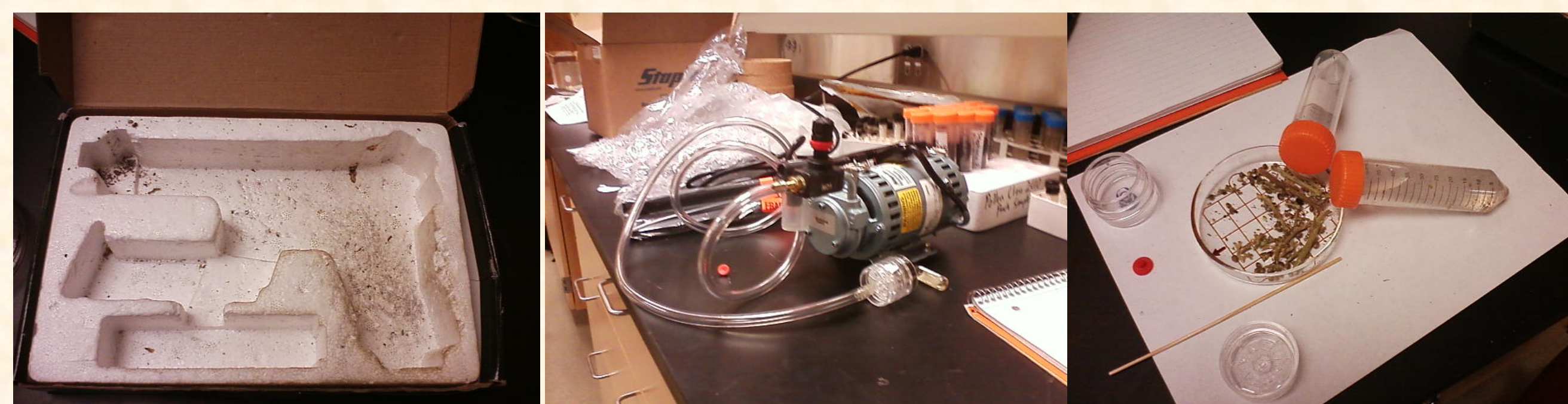
An air soft pellet gun box was used to store cannabis and paraphernalia (left); the lab vacuum used for pollen recovery (center); the vacuum filter was placed in a centrifuge tube for acetolysis once separated from larger debris (right).
