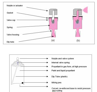
Figure 2. Internal arrangement of a paint spray can
