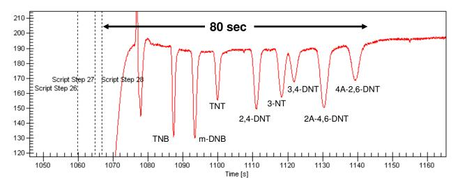
Figure 4: Separation obtained using an Agilent Bioanalyser 2100 platform. Electrolyte: 50mM SDS & 50mM Borate with 1.5% AgilentTM Dye (v/v).
