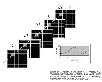
Figure 2: Schematic summarising the principles of chemical imaging. Light intensity is recorded as a function of both wavelength and location. The resulting data set can be seen as a full image at each  $\lambda$  or as a full spectrum at each pixel.
