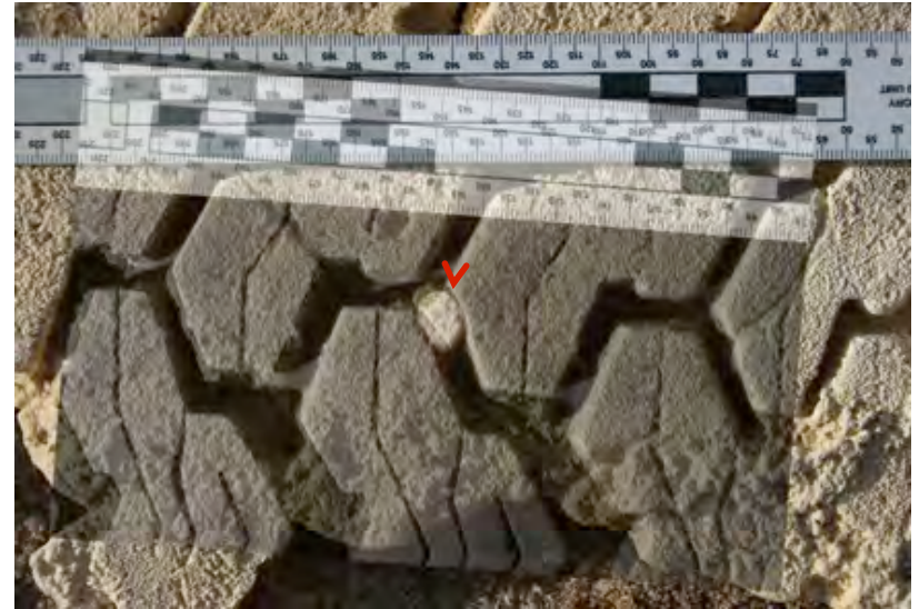
Photograph of segment of right rear tire overlaid on top of the cast to show correlation of stone hold.
